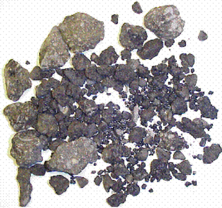
Figure 2.16: RAP in Aggregate-Sized Chunks
