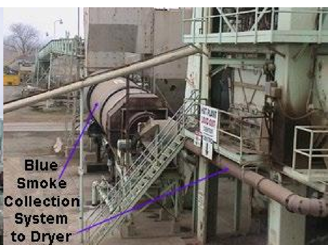
Induction Fan of Blue Smoke Collection System
