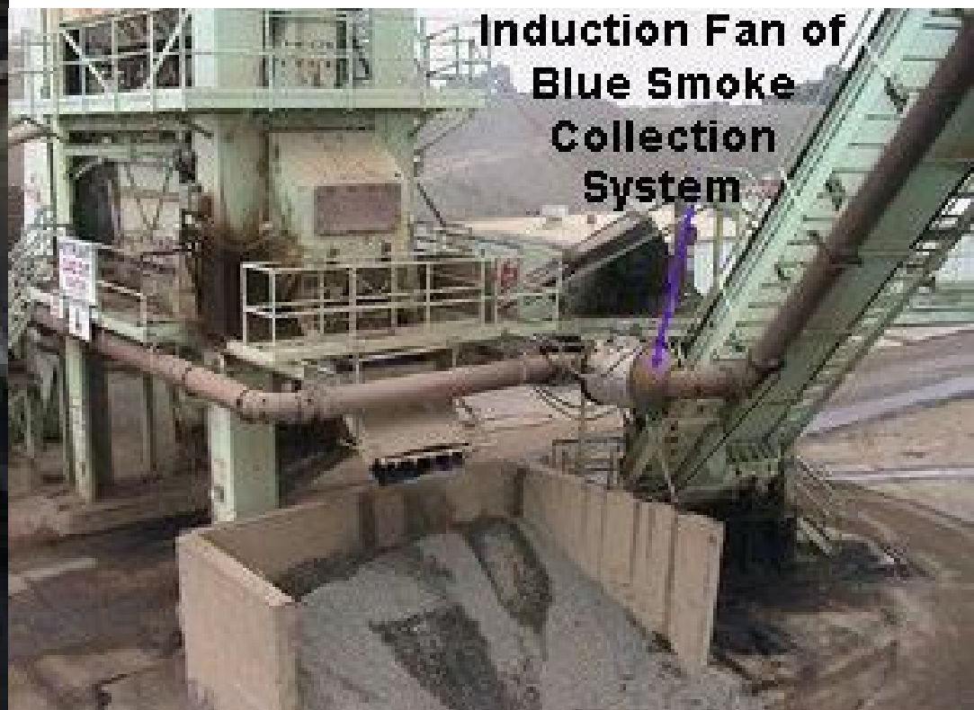
Blue Smoke Collection System to Dryer
