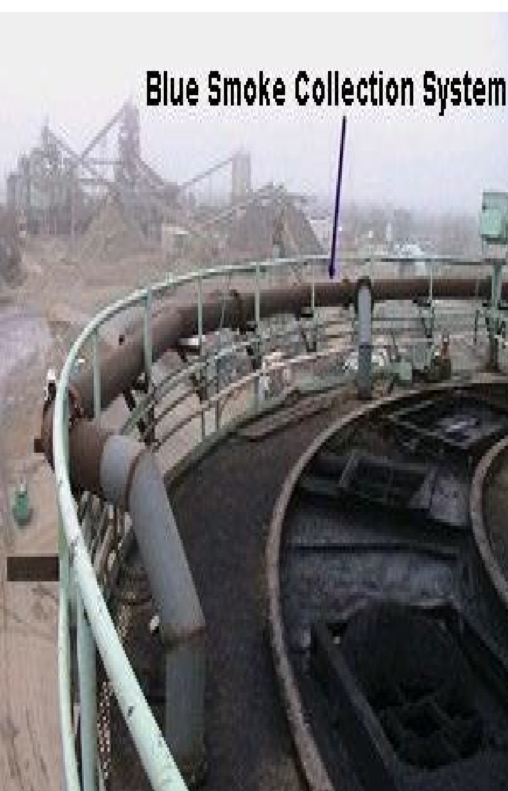
Blue Smoke Collection System to Dryer
